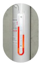
A common gauge found on radon mitigation systems is a U-tube filled with red liquid called a manometer or vacuum gauge.
