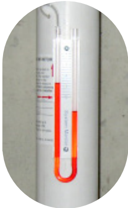
A common gauge found on radon mitigation systems is a U-tube filled with red liquid called a manometer or vacuum gauge.
